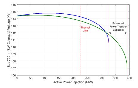
Stress the system by increasing generation and load *simultaneously* at *multiple* nodes until reliability issues, either thermal or transfer limits, are encountered:
