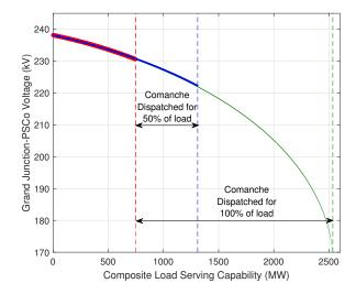
The power transfer capability between Colorado and the rest of the Western Interconnection is limited. How to mitigate this issue?
